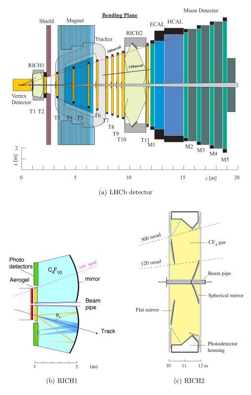
Figure 3.13: (a) The cross sectional view of the LHCb detector [49]. The LHCb detector has two RICH counters, RICH1 (b) and RICH2 (c) [50]. The RICH1 counter employs the combination of silica aerogels and  $C_4F_{10}$  gas radiators. The RICH2 counter employs  $CF_4$  gas radiator.
