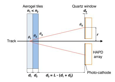
Figure 6.9: The schematic of the principle of Cherenkov angle reconstruction at the ARICH counter.  $d_i$  are thickness of each materials,  $\theta_1$  is the emission angle corresponding to  $\theta_{\rm C}$ , and  $\theta_i$  are refractive angle  $n_i$  at the *i*th material given by the Snell's law Eq.(4.1). The emission point  $z_e$  is assumed at the middle of  $d_1$ .
