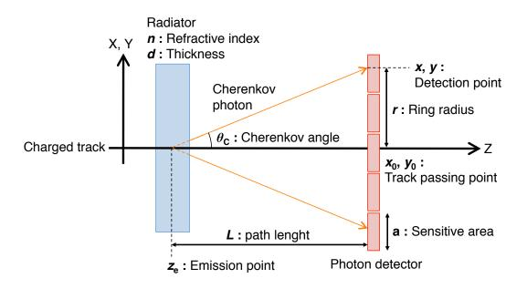
Figure 6.8: The schematic of the considerable parameters used for to determine of the Cherenkov angle resolution  $\theta_{\rm C}$ .
