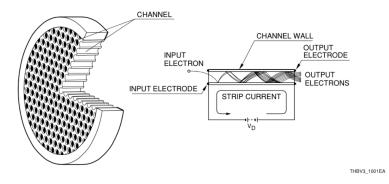
Figure 4.3: The schematics of the structure of a micro channel plate (MCP) [54]. Left: overview of the MCP. Right: the principle of the electron amplification in an MCP channel hole.
