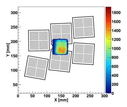
Figure 6.6: The beam profile on the surface of HAPD array.
