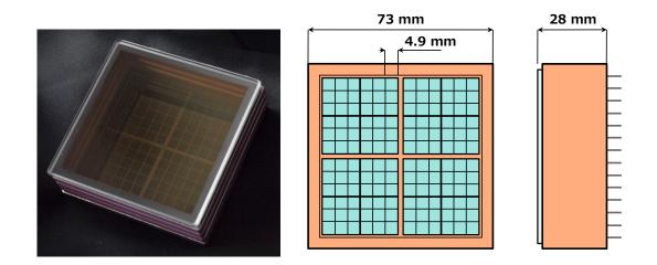
Figure 5.1: Picture of the exterior (left) and the design of the 144-ch HAPD (right).
