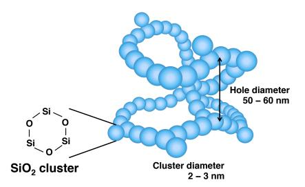
Figure 3.4: The illustration of three-dimensional networks of silica particles.  $SiO_2$  clusters become a primary particle with a diameter of 2–3 nm. They will connect each other three-dimensionally with hole-gap of 50–60 nm.
