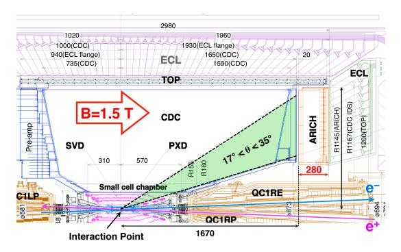
Figure 4.1: Horizontal cross-section of the Belle II detector. The ARICH counter will be installed in the forward end-cap region corresponding to the polar angle range  $17^{\circ} < \theta < 35^{\circ}$  from the interaction point (IP). Only 280 mm along the beam pipe direction is available for the ARICH counter, and a high magnetic field of 1.5 T exists in this region.
