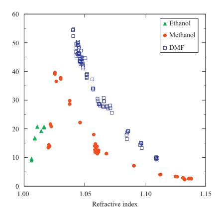
Figure 4.5: Transmission length as a function of the refractive indices at 400 nm of injected photons [36]. Markers are corresponding to kinds of a solvent used for synthesizing of alcogel with an ethanol (triangles), a methanol (circles), and DMF (squares), respectively.
