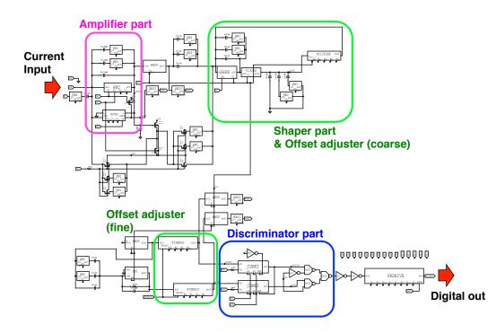
Figure 4.10: The block diagram of the SA03 main circuit of a channel.
