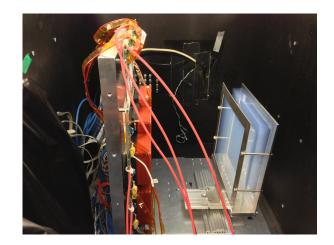
Figure 6.2: The photograph of the prototype ARICH counter in the light-tight box.
