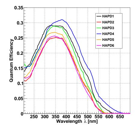
Figure 6.11: Quantum efficiencies of HAPDs mounted in the prototype ARICH counter as a function of wavelength [54].
