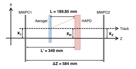
Figure 6.10: The schematic of the determination of the tracking resolution  $\sigma_{x_{\rm H}}$ .
