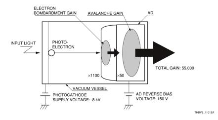
Figure 4.4: The schematics of the structure of a Hybrid Photo detector (HPD) [54].
