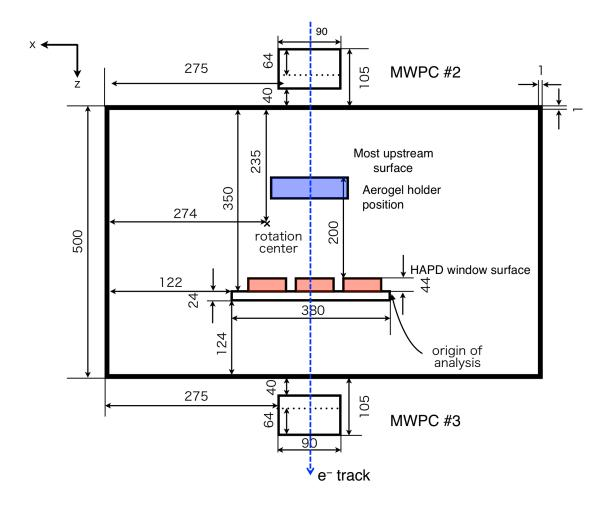
Figure 6.4: The top view of the experimental setup of beam test
