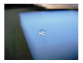
Figure 3.5: Picture of an aerogel tile with a low refractive index (n = 1.009) and hydrophobic [36]. This aerogel was produced using the recently in vented production method.
