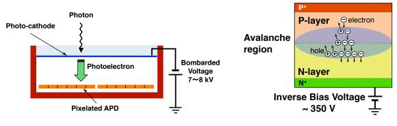
(a) A cross-sectional view of the HAPD (b) A illustration of the structure of an APD
