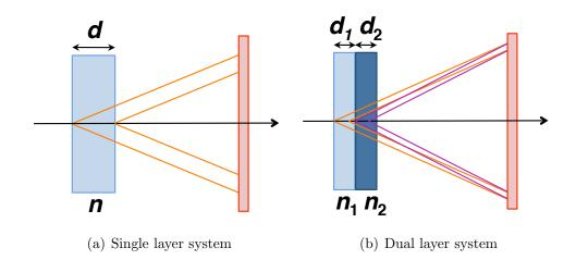
Figure 4.7: Schematics of proximity focusing schemes; (a) Normal type proximity focusing system with a single-layer radiator, (b) Proximity focusing system with dual layer focusing, which consists with different refractive indices of  $n_1$  and  $n_2$  ( $n_1 < n_2$ ) are used. The total thickness of aerogels d in both systems are the same.
