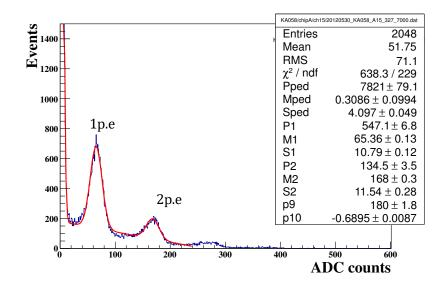
Figure 5.4: The pulse height distribution for low intensity pulsed LED illumination.
