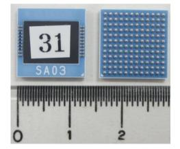
Figure 4.9: The picture of the ARICH readout ASIC (SA03): the front-side view (left) and the rear-side view (right).
