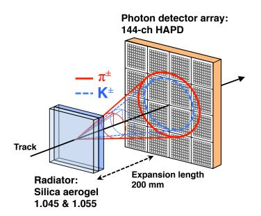
Figure 4.2: The conceptual design of the ARICH counter. The dual silica aerogel layer as the radiator and the 144-ch Hybrid Avalanche Photo Detectors as the photon detector will be used for this counter.
