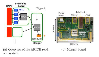
Figure 4.12: The schematic of the ARICH readout system (a) and the merger board (b).
