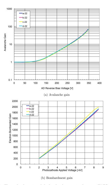
Figure 5.3: The avalanche gain and the bombardment gain of a recent HAPD sample. (a) Avalanche gain as a function of the applying inverse bias voltage. (b) Electron bombarded gain as a function of the bombardment voltage applying in photo-cathode.
